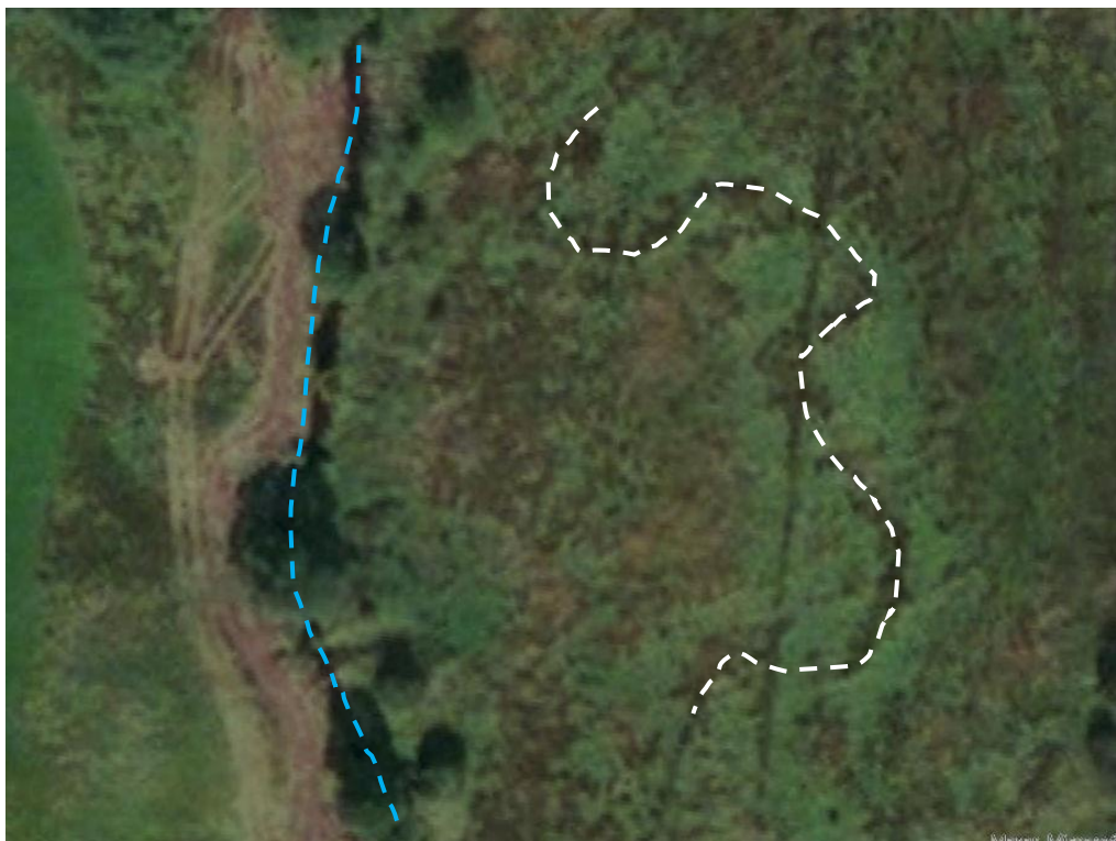
Figure 5. Clear signs of a naturally sinuous channel (white dashed line), evident by rushes and a wet area remaining in the field alongside the current straightened channel of the River Strade (blue dashed line). This area was not inspected in person but was identified from aerial photography maps. Similar can be found elsewhere all over the catchment.
